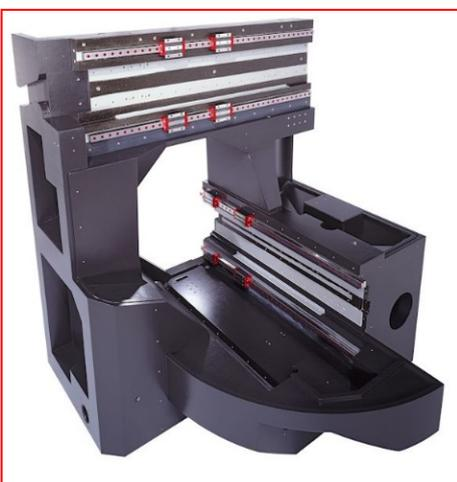
Exceptional dynamics from sustainable and environmentally friendly production – the machine bed of a high-speed milling machine made from RAMPF's EPUMENT mineral casting, with high-precision replicated surfaces manufactured using non-cutting processes for mounting guide rails, measuring systems, and drive components.
